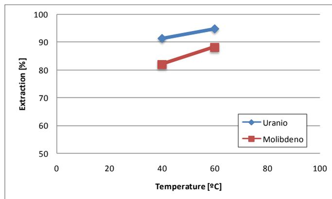
Figure 3. Process temperature tests (53% w/w).
