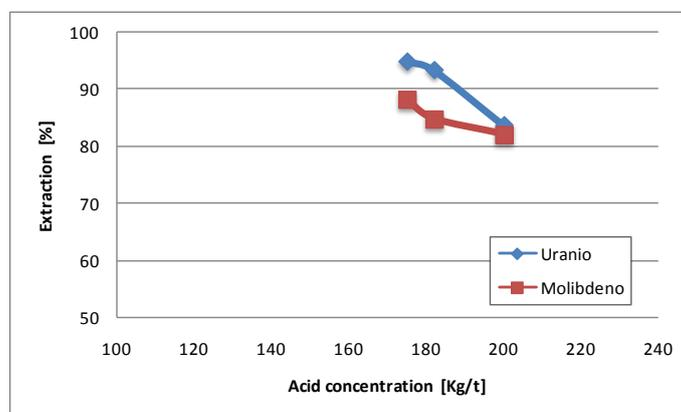
Figure 1. Acid concentration tests (53% w/w), 20 Kg/t MnO<sub>2</sub>, 60°C.
