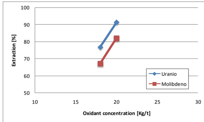
Figure 2. Oxidant concentration tests (53% w/w), 175 Kg/t  $H_2SO_4$ ; 40°C.
