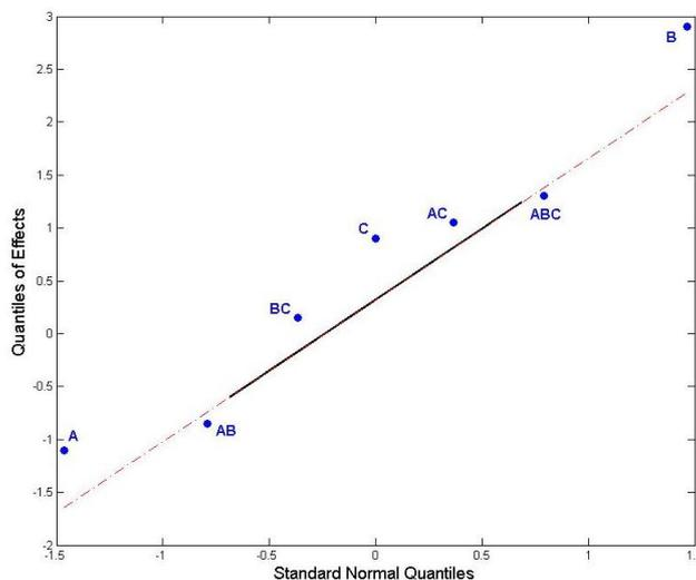
Figure 5. Normal probability plot of the effects for molybdenum extraction performed tests.
