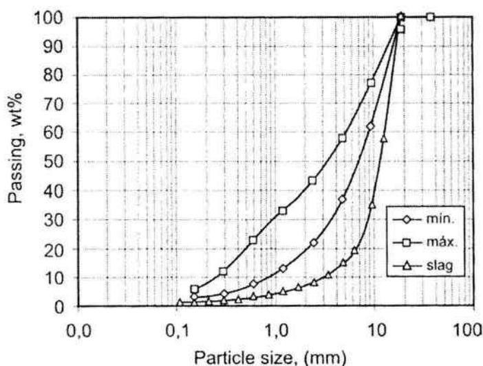
Figure 3. Particles size distribution of the total sample of copper slag compared with the Chilean standard NCh 165. Of 77 (1977).
