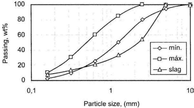
Figure 2. Particles size distribution of the sand fraction of the copper slag compared with the Chilean standard NCh 165. Of 77 (1977).
