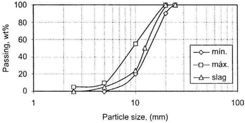
Figure 1. Particles size distribution of the coarse fraction of the copper slag compared with the Chilean standard NCh 165. Of 77 (1977).
