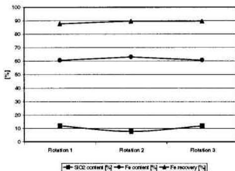
Figure 6: SiO<sub>2</sub> content, Fe content and Recovery of Fe for a 3-step flotation with the recycling of amines two times
