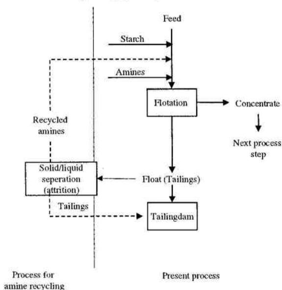
Figure 1: Present process of reverse iron ore flotation including the feasible process of amine recycling
