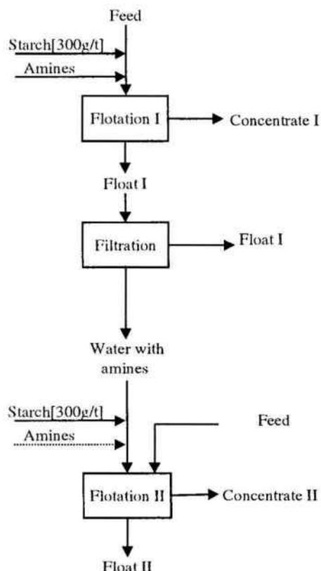
Figure 2: Course scheme of the flotation tests
