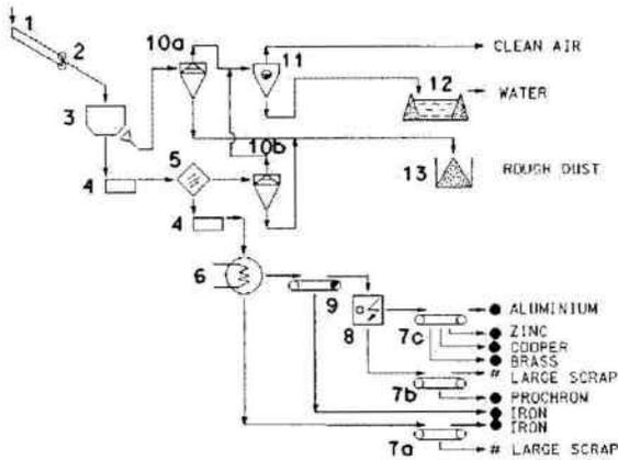
Fig. 3 Segregative flowsheet of metallic scrap processing
