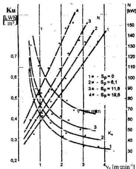
Fig. 1. Power consumption  $N$ , and unit energy consumption index  $K_u$  as a function of the heading machine advance for the four values of tip's blunt  $S_p$
