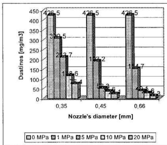
Fig.3. Dustiness by machining of an artificial concrete sample with a longitudinal experimental organ as a function of jet's pressure and nozzle's diameter
