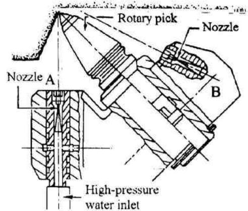
Fig.2. Scheme of possible supports for rotary pick by use of a high-pressure water jet
