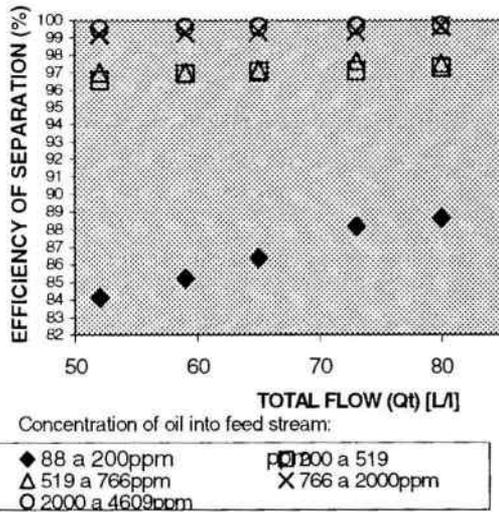
Figure 2 - Efficiency of separation as function of total flow to several oil concentration into feed.
