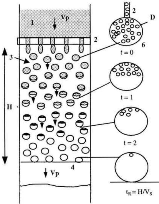
Figure 1 - Phase inversion principle.
