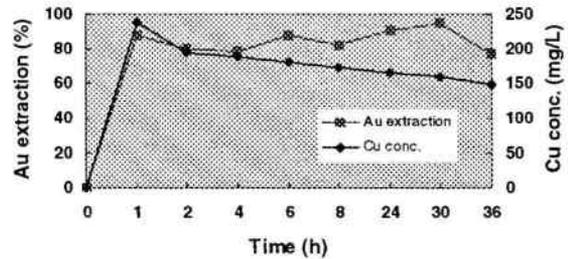
Figure 4 - Kinetics of gold extraction and copper leaching with air under optimal conditions
