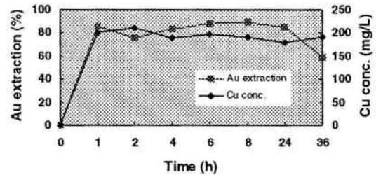
Figure 3 - Kinetics of gold extraction and copper leaching with O<sub>2</sub> under optimal conditions
