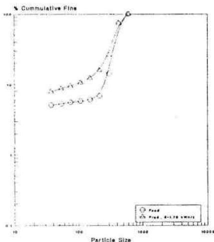
FIGURE 9. Effect of Fine Feed Size
