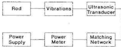
FIGURE 1. Schematic Diagram of The Ultrasonic Nip Roll Grinder at The USA Comminution Center.
