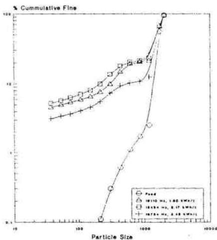
FIGURE 3. Effect of Frequency on Energy Consumption and Product Size Distribution.
