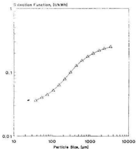
FIGURE 6. Specific Selection Function for a Chilean Copper Ore in a 18'x 24' (DxL) Ball Mill.
