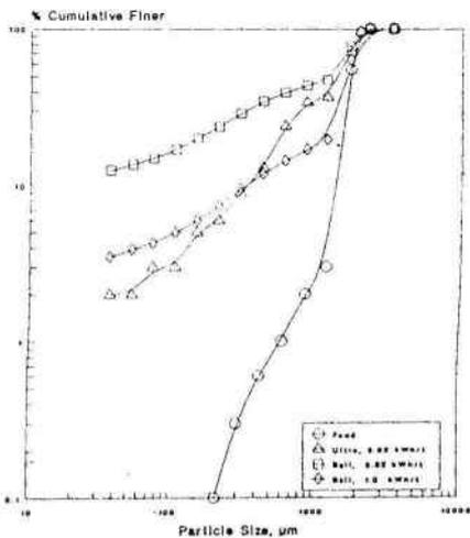
FIGURE 8. Comparison to Scaled-Down Ball Milling and Experimental Ultrasonic Nip Roll, Gap = 130  $\mu\text{m}$ .
